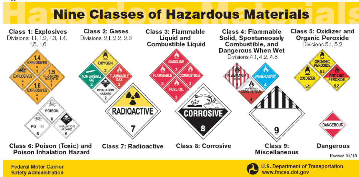
Figure 4-19: Hazardous Materials Classes
